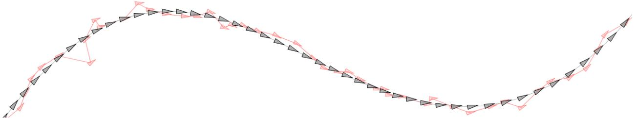
**Figure:** A sequence of noisy localization estimates of a fast driving go-kart in red, and the result of smoothing in black. ■
