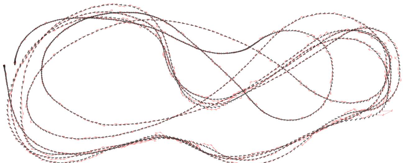
**Figure:** Sequence of vehicle pose estimates of a fast driving go-kart in red. The result of applying the smoothing filter is indicated in gray. ■
