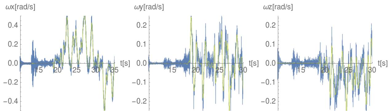
**Figure:** The orientation components of the discrete differences before (blue) and after the smoothing (yellow) during the time 10 – 35[s]. ■
