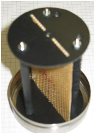
The inner structure is based on circular plastic plates that are attached to three cylindrical rods. The rods are also made of stainless steel, and are composed of smaller screw-together rods. The rods will be covered in plastic tape for isolation. Two rectangular slits on each of the plates, and a fitting contour of the circuit board, keeps the circuit board in place. The rods do not make contact with the circuit board.
